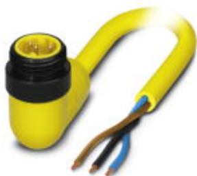
Power cable, 3-position, PVC, yellow, Plug angled 7/8"-16UNF, A - standard, on free cable end, cable length: 2 m
